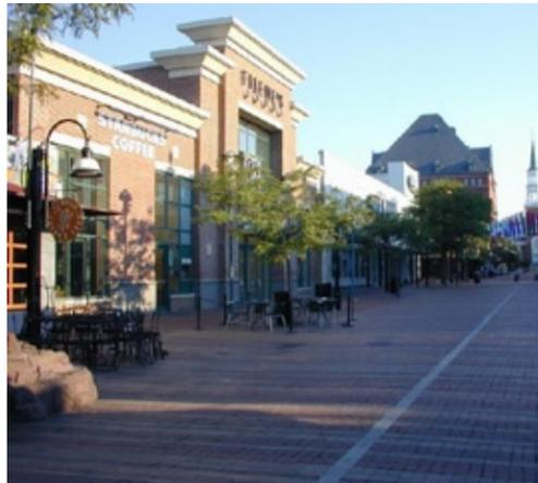
For example, a 100-foot wide roadway right-of-way should be framed by buildings that are at least 25 feet high (a typical two-story building) on both sides with facades that are at most 20 feet from the edge of right-of-way.
