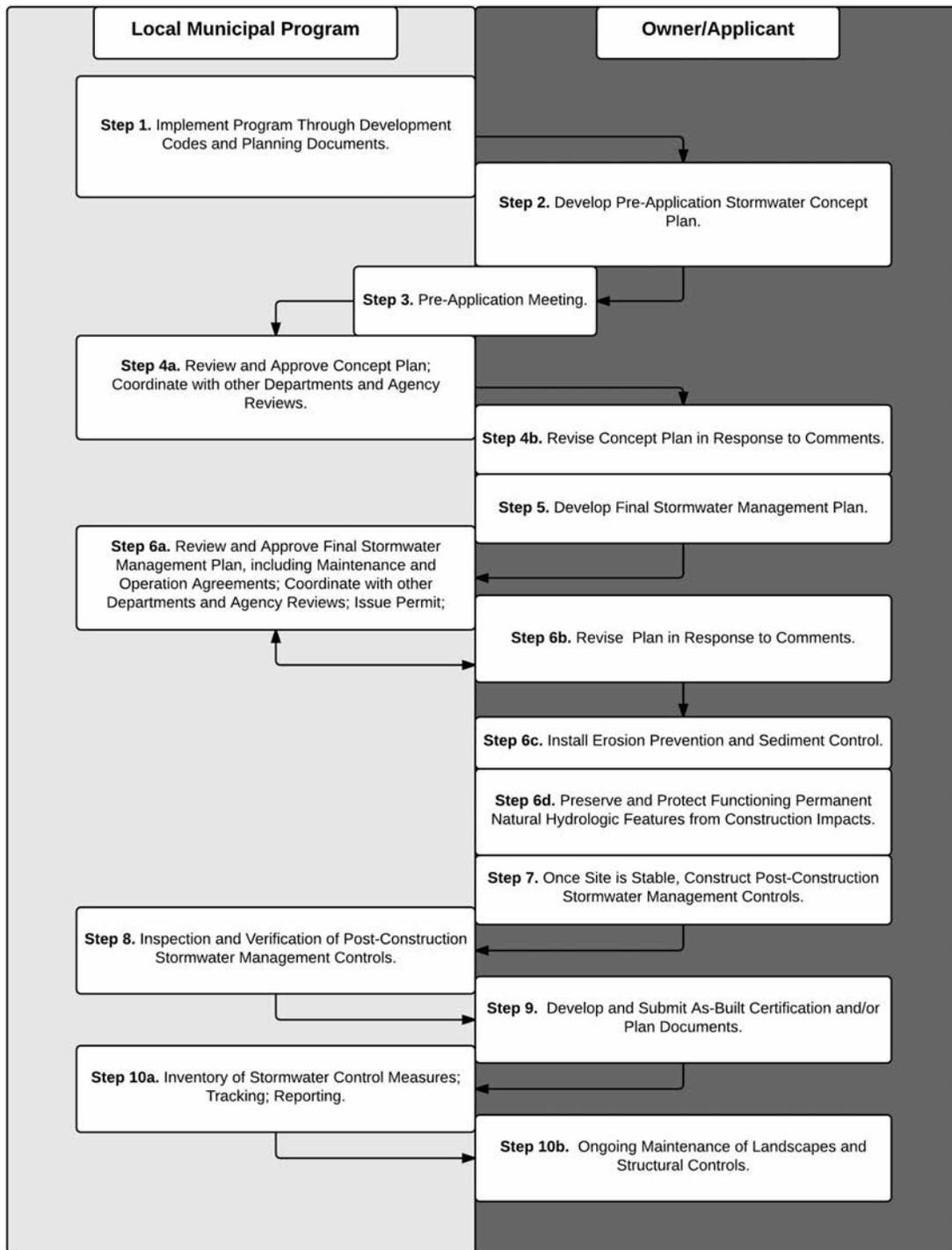
**Figure 2.6: Typical Compliance Pathway for Permanent Stormwater Runoff Management for New Development and Redevelopment Projects.**
