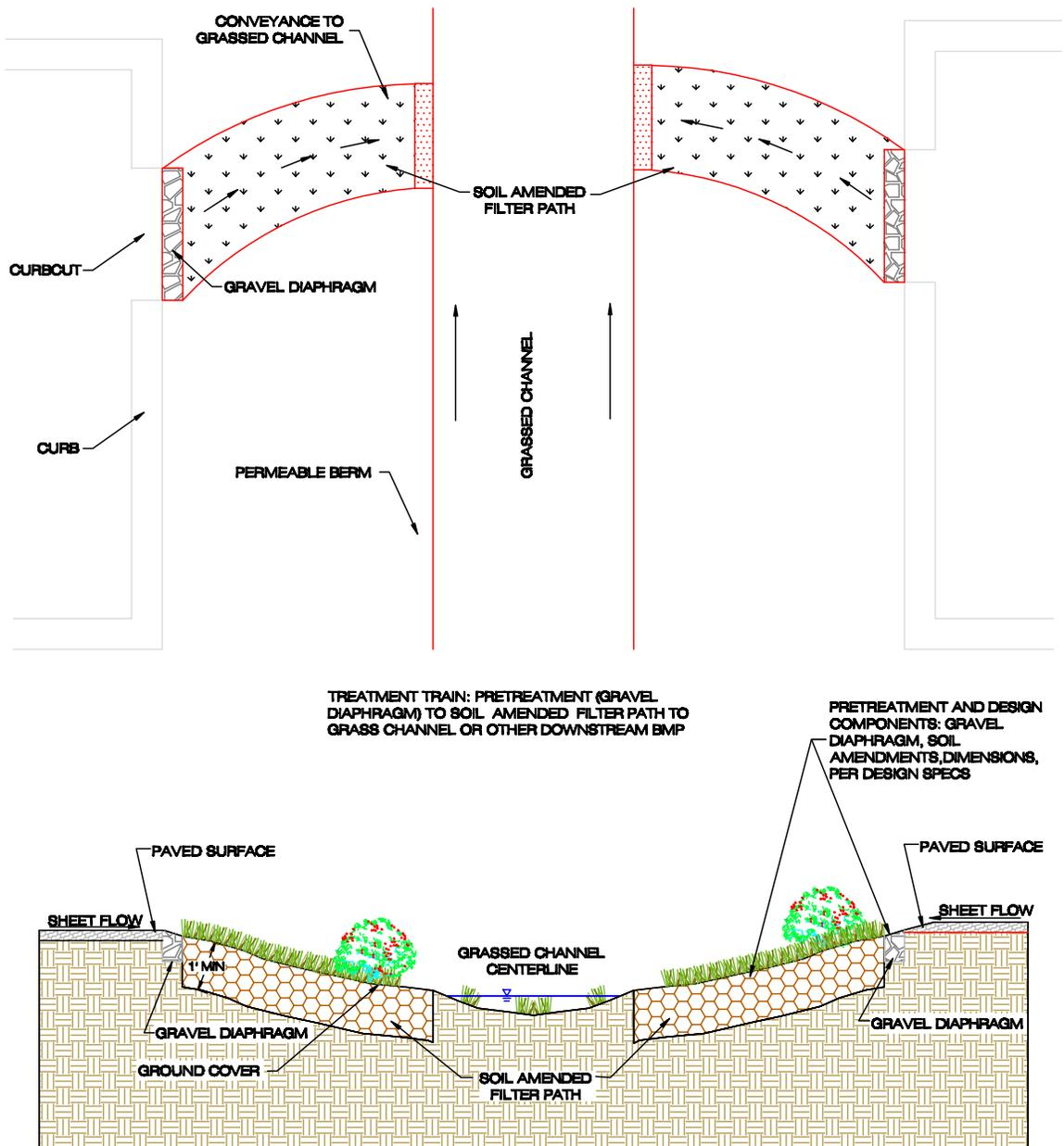
Figure 8: Filter path to grass channel (Source: Virginia).
