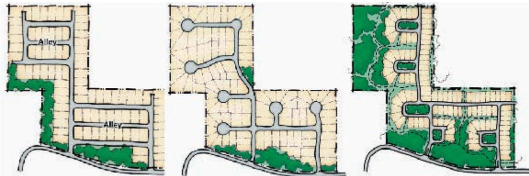
Figure 3.6: From left to right: grid, curvilinear, and hybrid pattern (AHBL Engineering).
