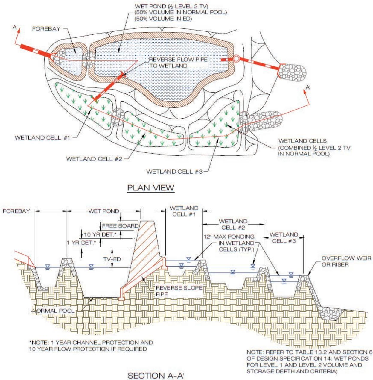
Figure 5: Pond-Wetland Combination – Plan and Section.
