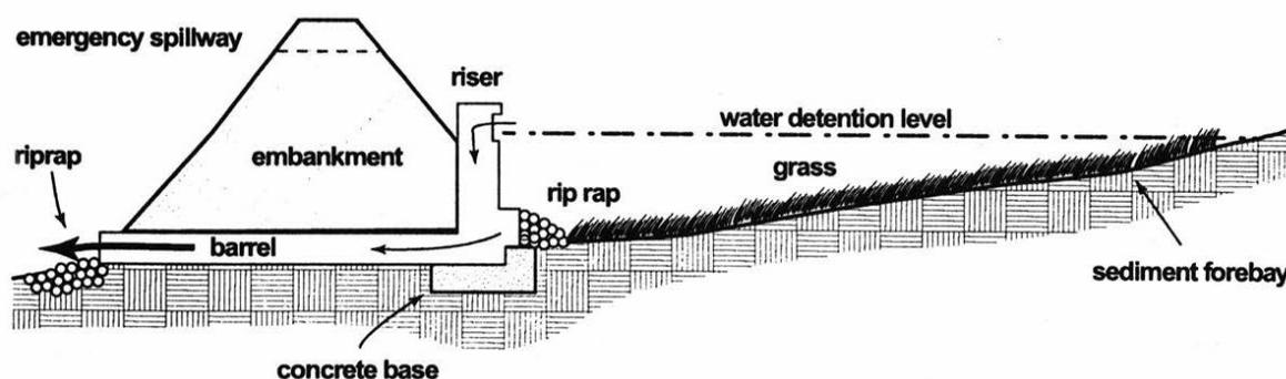
Figure 2: Dry detention pond cross-section (US EPA).
