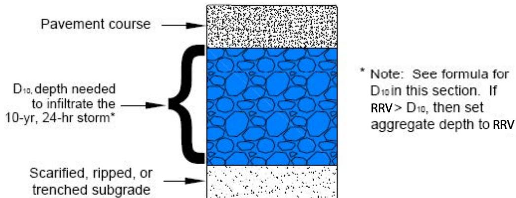
Figure 5: Infiltrate the 10-yr, 24-hr storm (Source: NCSU-BAE).
