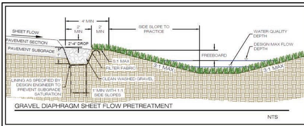
Figure 6: Pretreatment option – gravel diaphragm for sheet flow (Source: VADCR).
