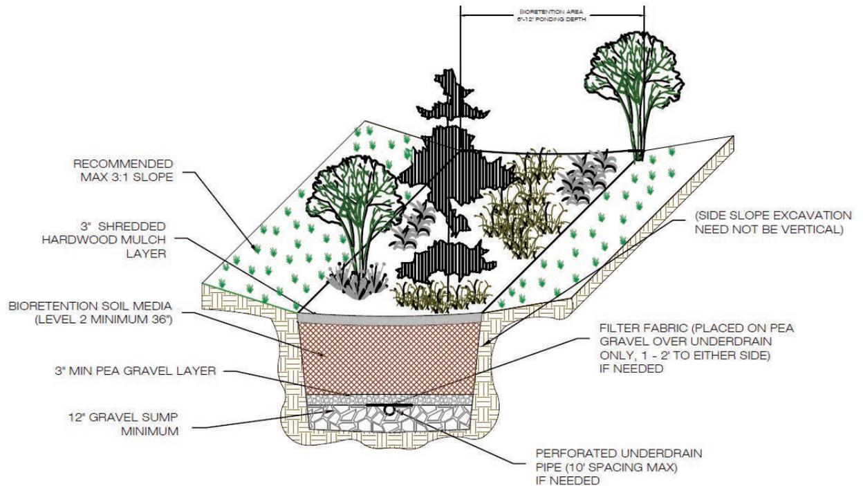
Figure 19: Typical section with underdrain (Source: VADCR).
