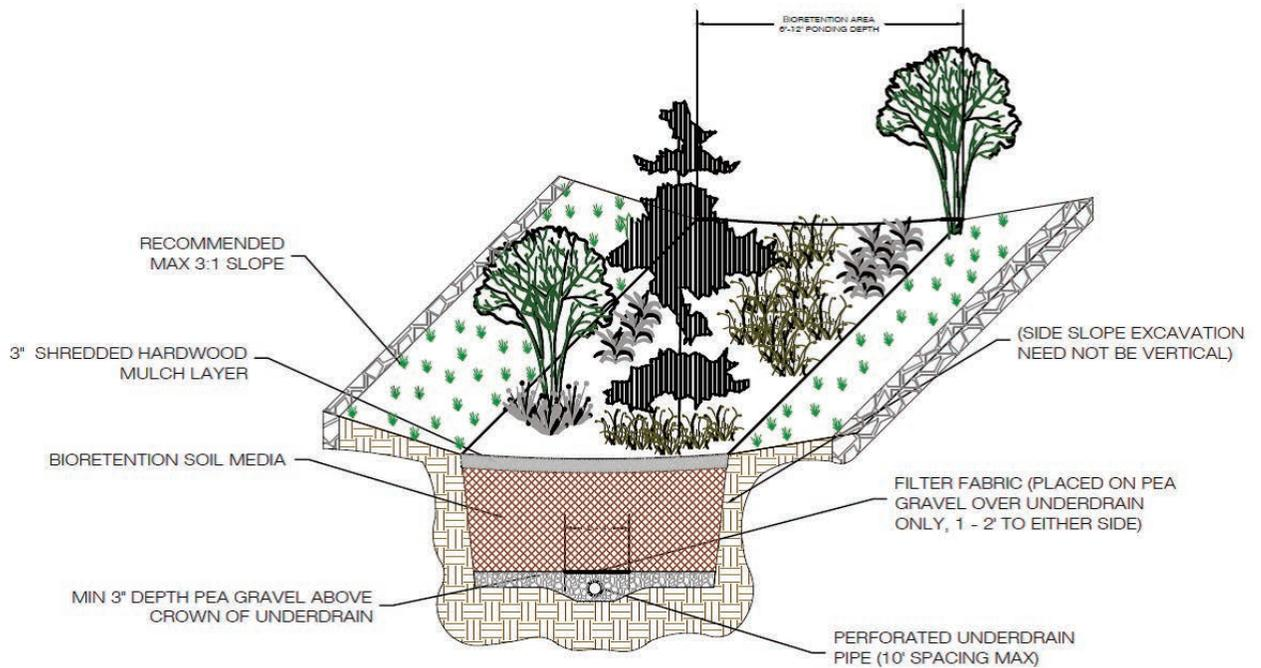
Figure 18: Typical section with underdrain (Source: VADCR).
