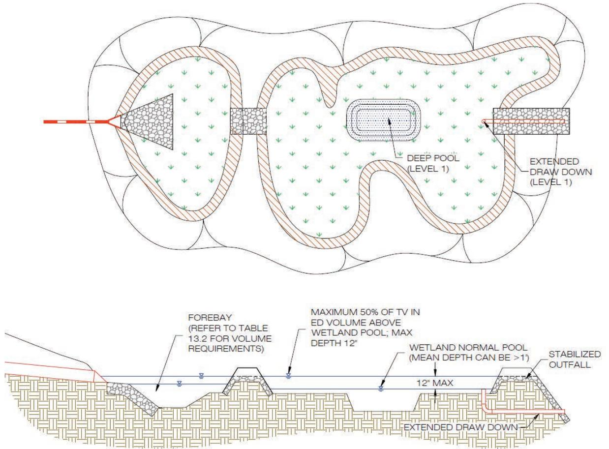
Figure 4: Constructed Wetland Plan and Cross Section.
