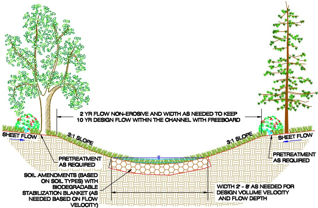
Figure 6: Grass swale with compost amendments – sections
