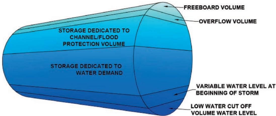
**Figure 7: Incremental Design Volumes associated with tank sizing**
