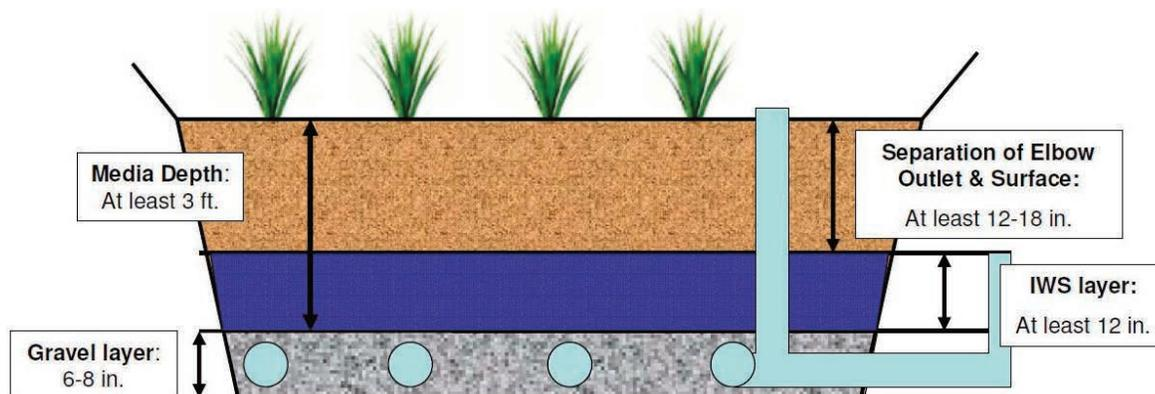
Figure 11: Bioretention cell showing IWS zones (Source: NCDENR).
