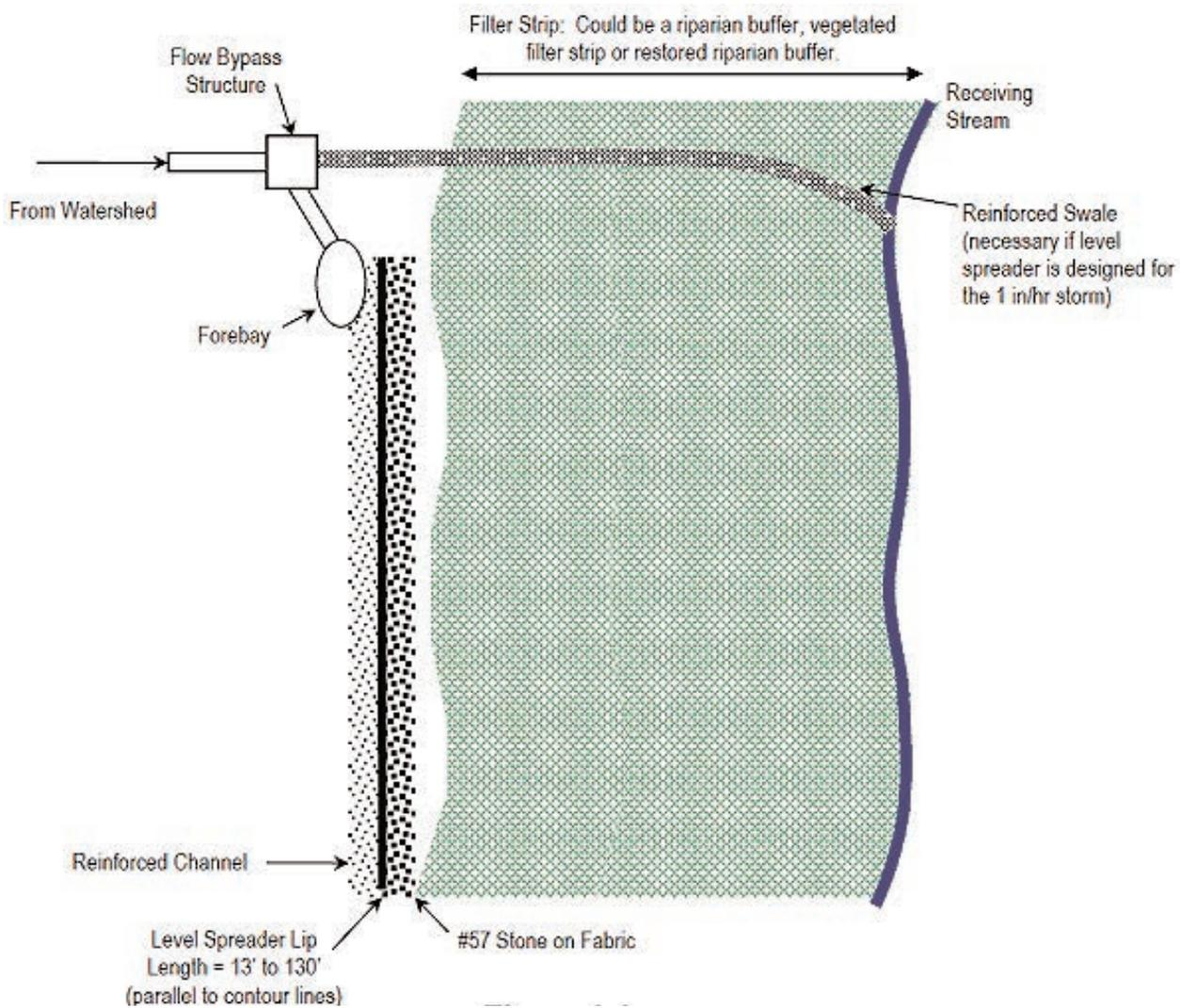
Figure 3a: Engineered Level Spreader (ELS) Plan (Hathaway 2006).
