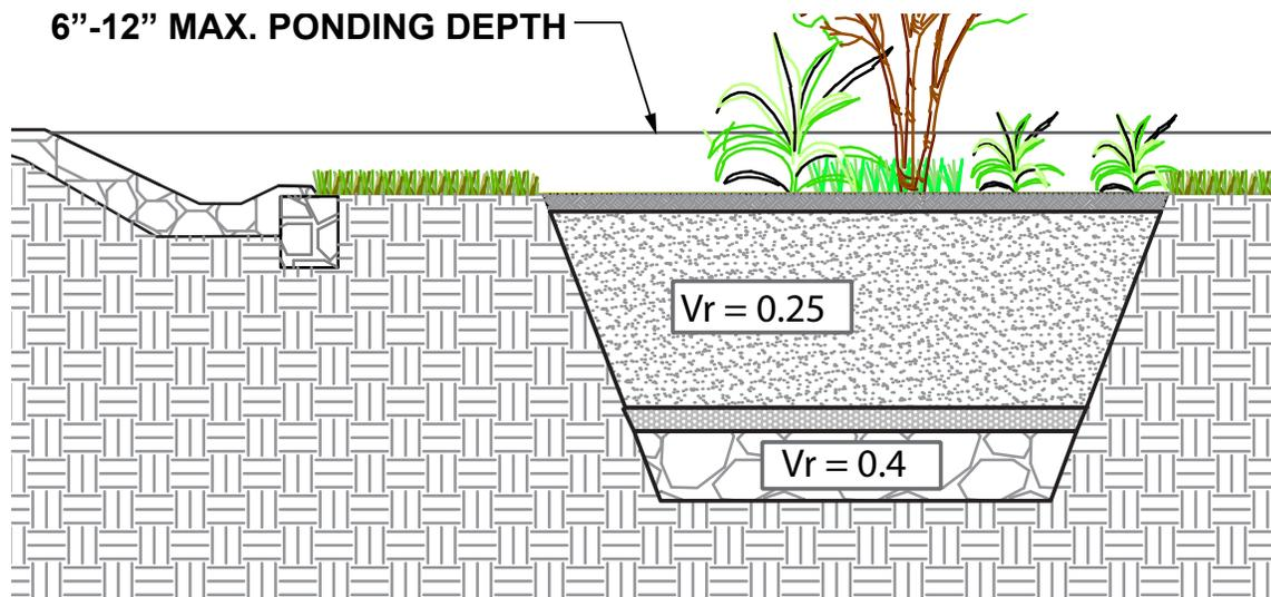
Figure 14: Typical bioretention section with void ratios for volume computations
