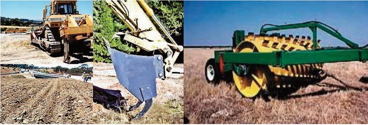
**Figure 5.5: Attachments used for soil decompaction.**
