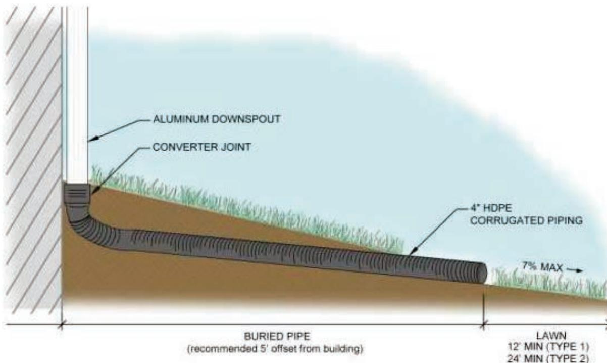
**Figure 5c: Buried pipe outlet configuration (Source: Carmen, NCSU).**
