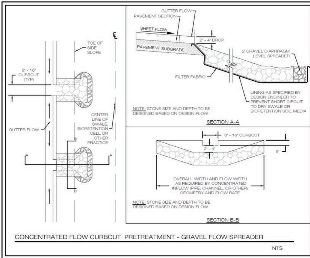
Figure 7: Pretreatment – Gravel from spreader for concentrated flow
