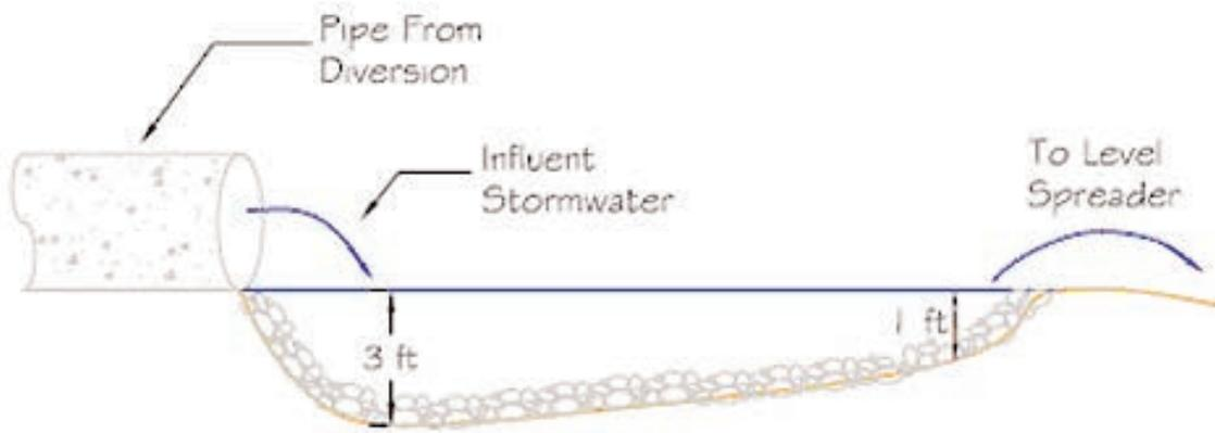
Figure 2: Level Spreader Forebay (Hathaway and Hunt 2006).
