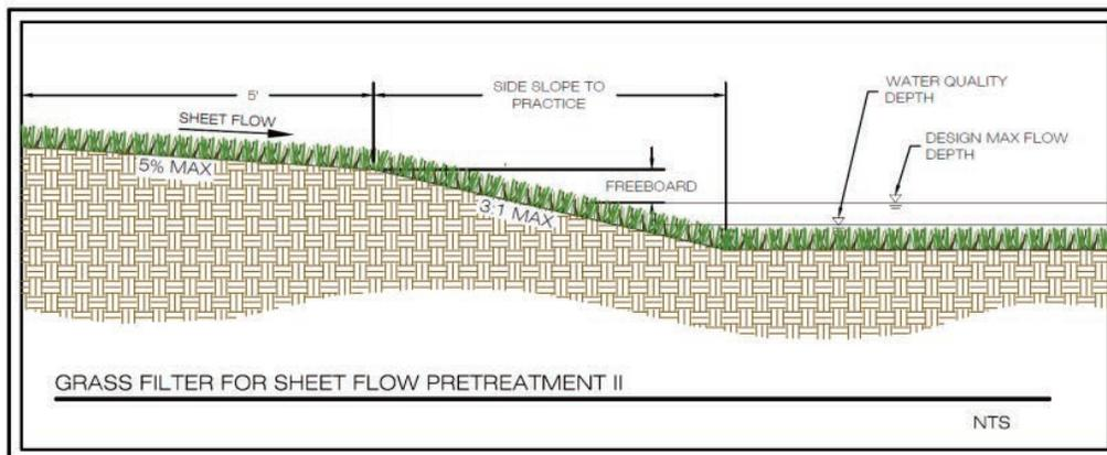
Figure 5: Pretreatment option – grass filter for sheet flow (Source: VADCR).
