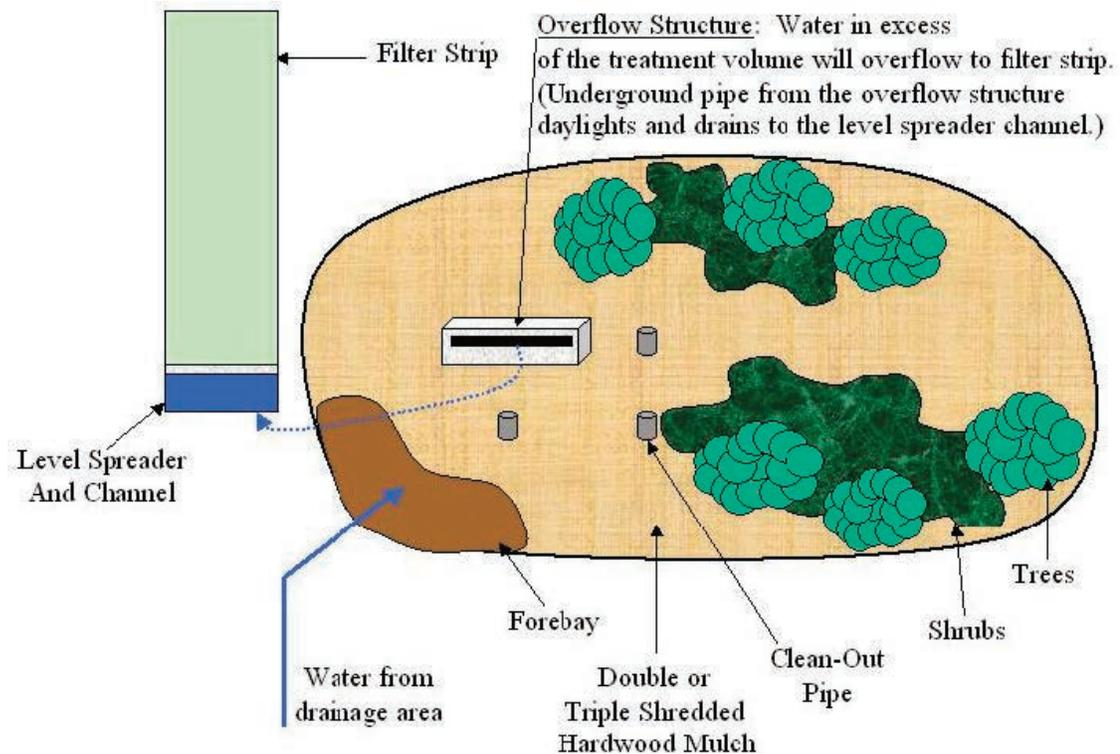
**Figure 12:** Bioretention units can be designed using an overflow device so that water in excess of the treatment volume overflows to a filter strip. This example shows a filter strip, though it is not required for every design (Source: NCDENR).
