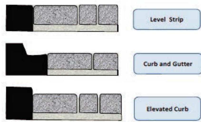
Figure 12: Examples of perimeter edge restraints (Source: NCDENR).
