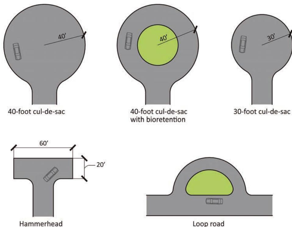
Figure 3.7: Various road designs. (adapted from Schueler, 1995).
