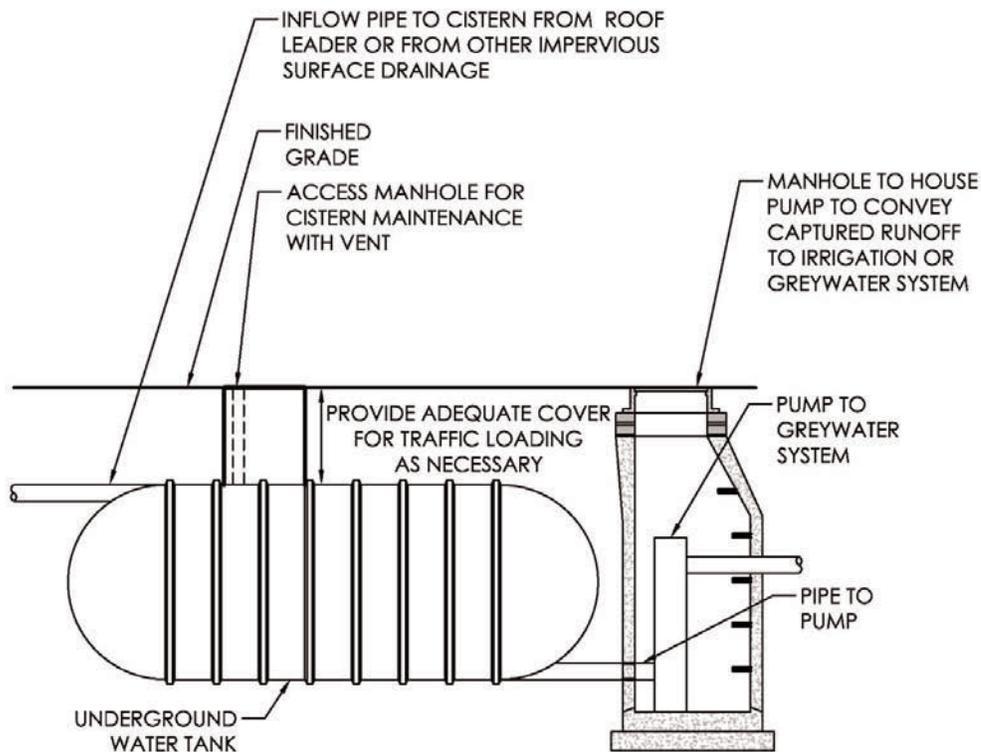
**Figure 5: Cross-section of an underground cistern (Source: CHCRPC).**
