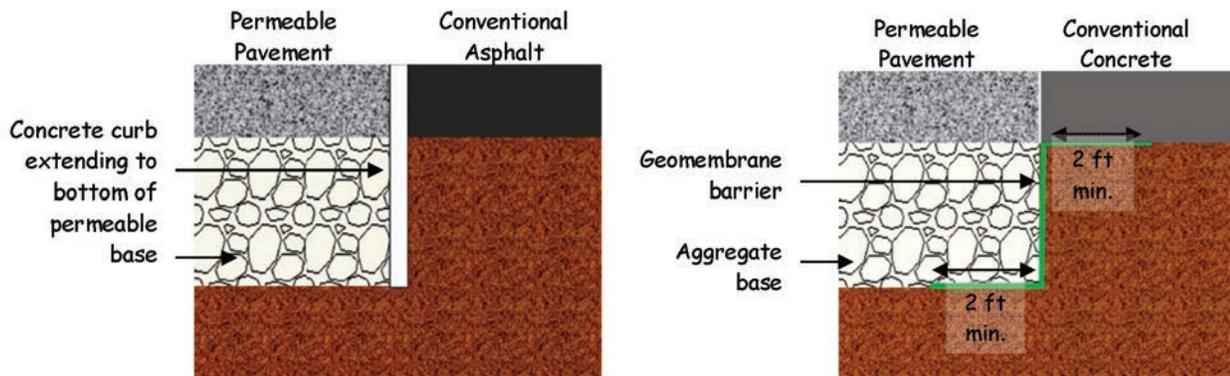
Figure 13: Detail of separation between permeable and conventional pavement (Source: NCDENR).
