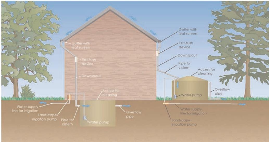
**Figure 4: Roof runoff can be captured in cisterns above or below grade and used for irrigation or non-potable water needs (Source: CHRPC, 2012).**
