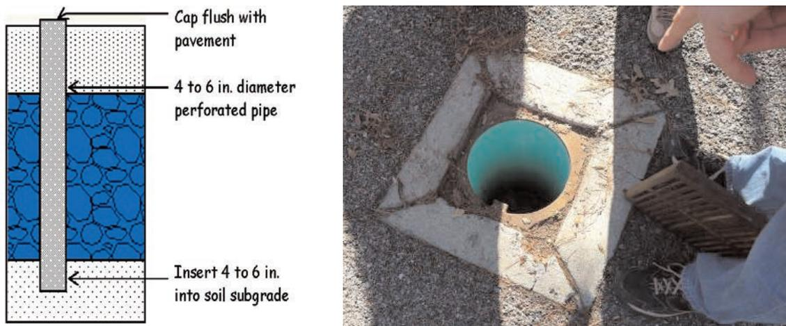
Figure 10: An observation well enables inspection of water infiltration (Source: NCDENR).
