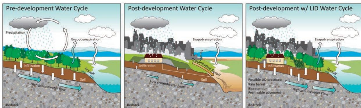
**Figure 2.4: Comparison of the natural and urban water cycles and a depiction of how low impact development creates opportunities in the urban environment to mimic the natural cycle (modified from The Auckland City Council, 2010).**
