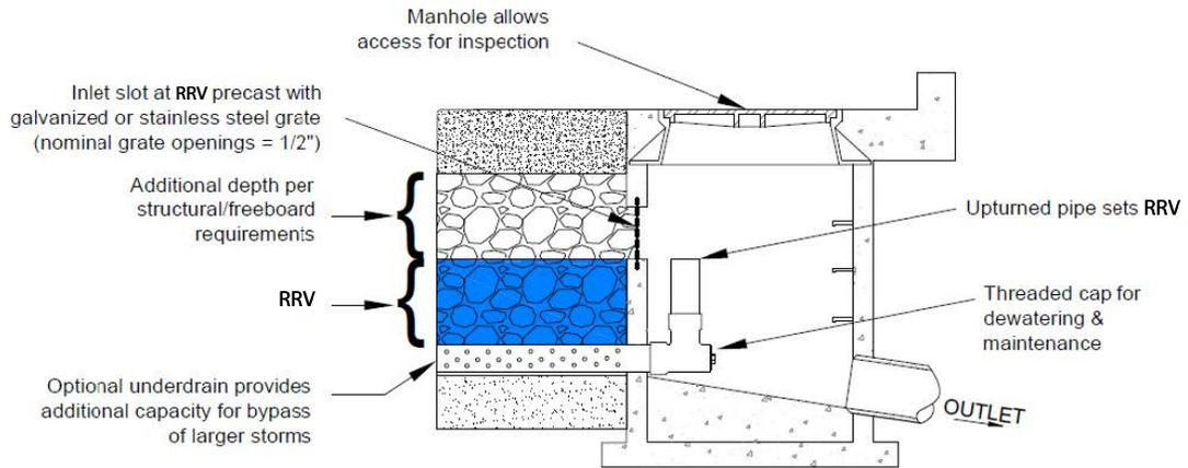
Figure 7: Bypass via subsurface openings in manhole structures (Source: NCSU-BAE).
