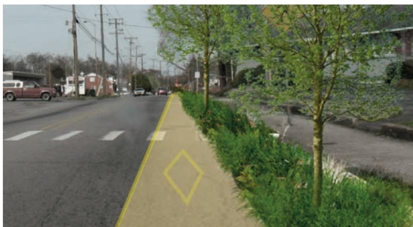
**Figure 3.10: Some street retrofitted with linear bioretention, bike lane,
