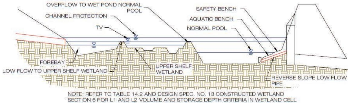
NOTE: REFER TO TABLE 14.2 AND DESIGN SPEC. NO. 13 CONSTRUCTED WETLAND SECTION 6 FOR L1 AND L2 VOLUME AND STORAGE DEPTH CRITERIA IN WETLAND CELL
