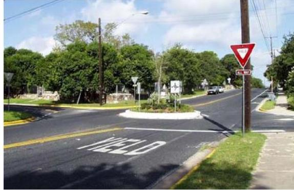
*Figure 6 A traffic circle creates a horizontal deflection in the roadway, which causes motorists to slow down as they travel through the intersection*
