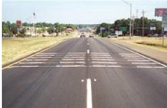
*Figure 4 Rumble Strips are typically used to alert motorists of unusual conditions, like crosswalks.*
