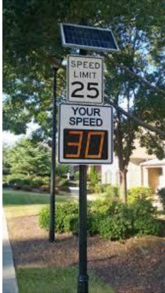
*Figure 2 Solar radar speed limit signs may help to reduce speeds by up to 20%.*
