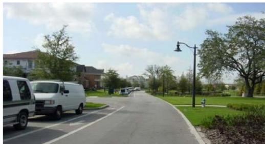
*Figure 3 The addition of a bike lane on this street helps to create a narrow travel lane for motorists.*
